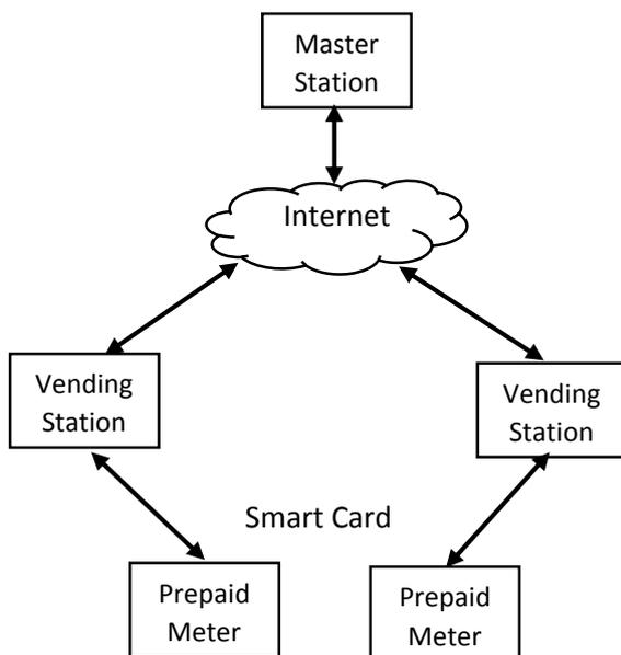
Figure 1: Architecture of the Prepaid Metering System
