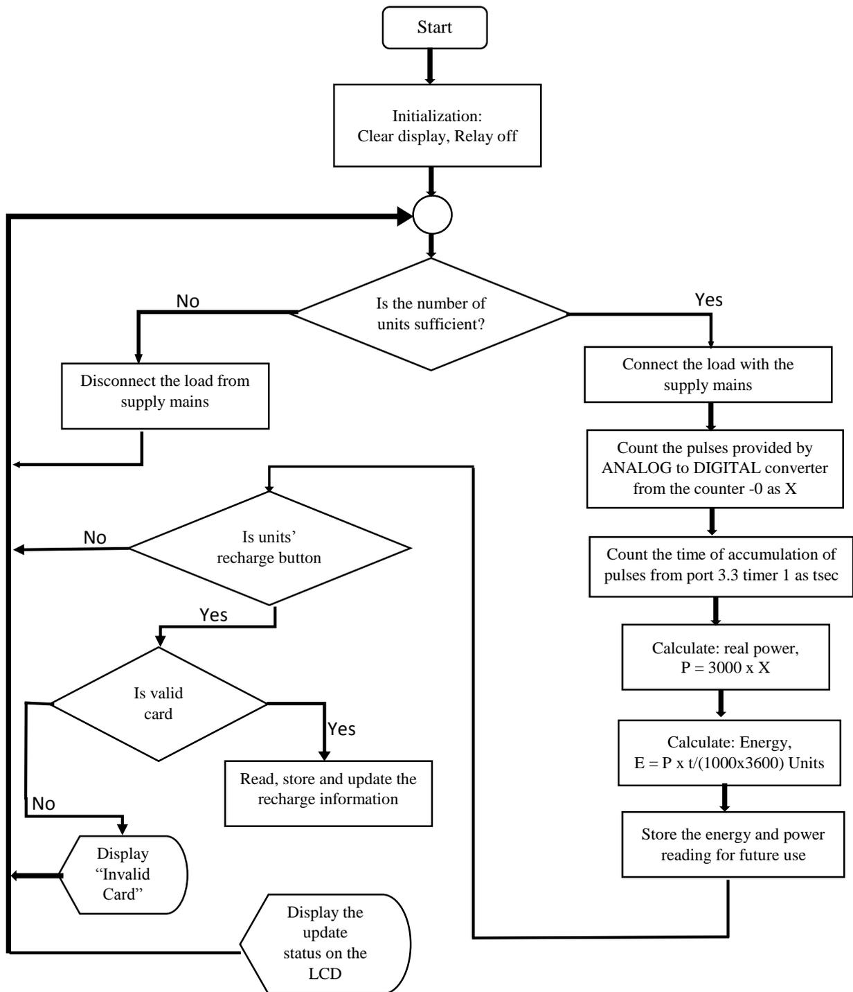
Figure 4: Flowchart of Prepaid Smart Card Energy Meter
