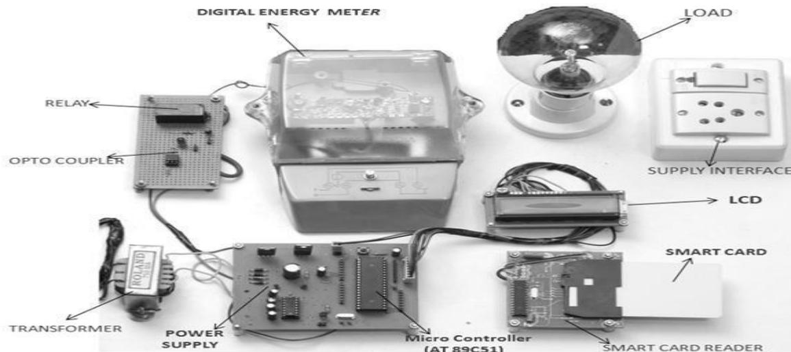
Figure 3: Designed and Implementation of Prepaid Smart Card Energy Meter
