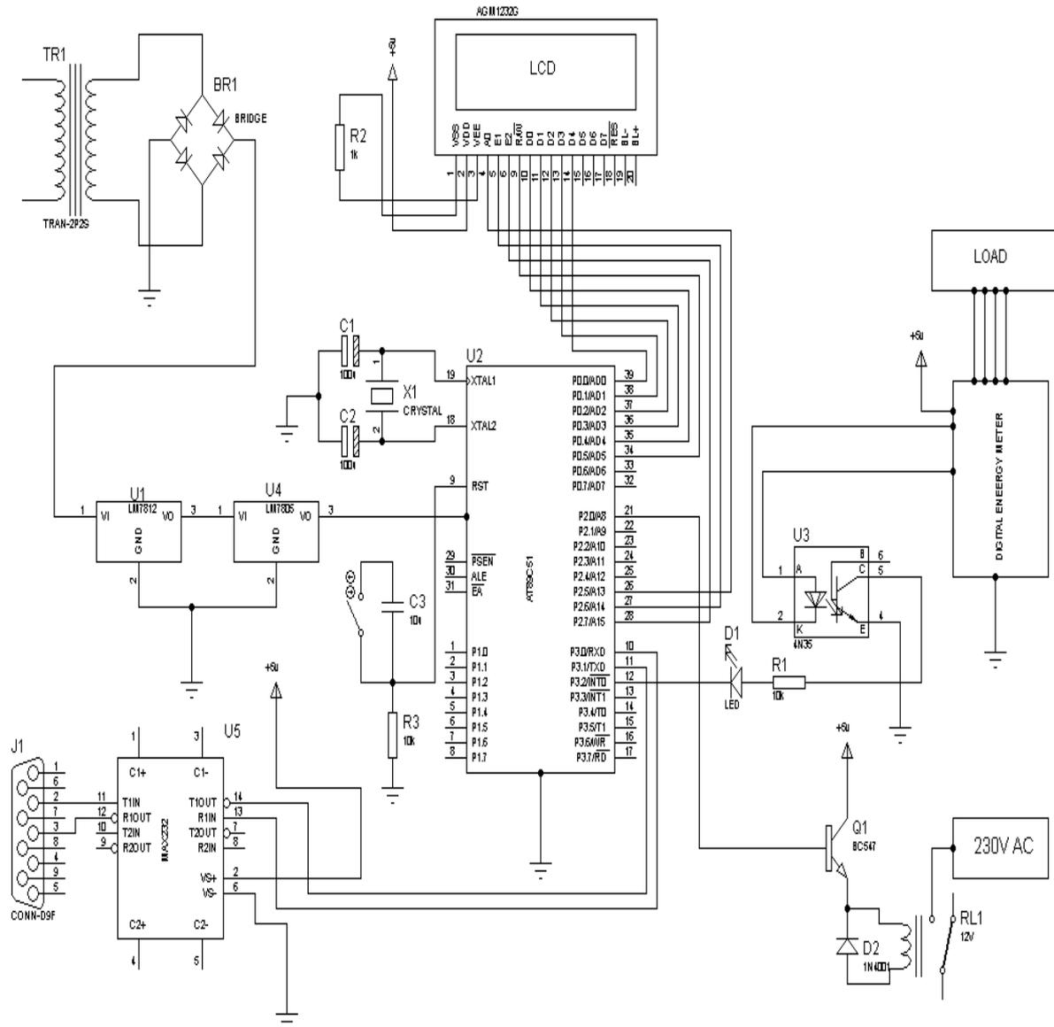
Figure 2: Circuit diagram of Prepaid Smart Card Energy Meter
