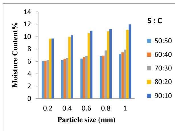
Figure 8: Effects of binder, mixing ratios and particle sizes on moisture content for briquettes sample B (orange waste)
