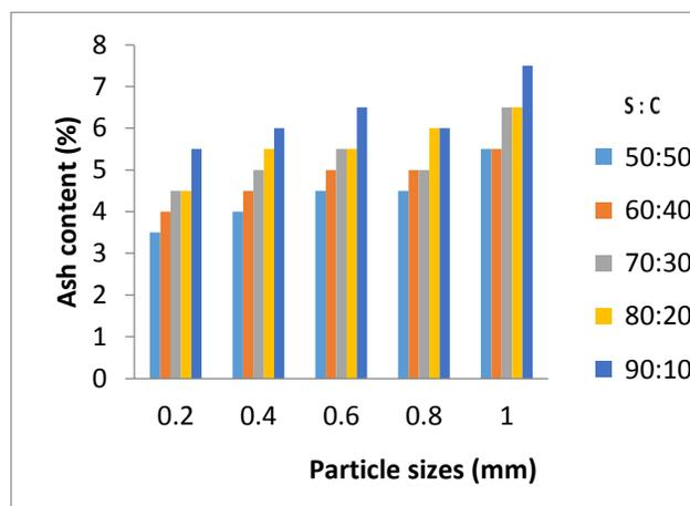
Figure 9: Effects of binder, mixing ratios and particle sizes on ash content for briquettes sample A (cassava starch gel)
