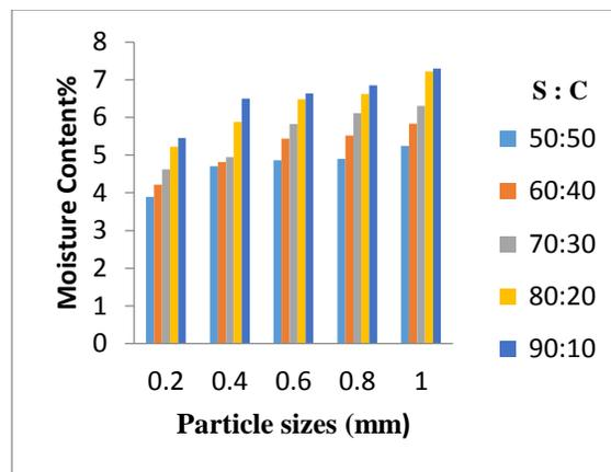
Figure 7: Effects of binder, mixing ratios and particle sizes on moisture content for briquettes sample A (cassava starch gel)
