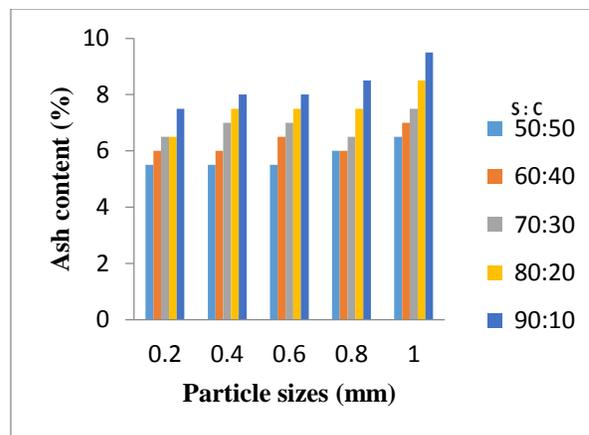
Figure 10: Effects of binder, mixing ratios and particle sizes on ash content for briquettes sample B (orange waste)
