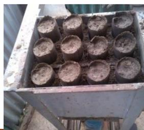
Figure 6: Moulding of briquettes
