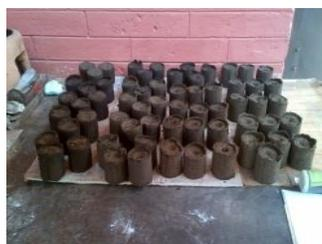
Figure 5: Briquettes produced
