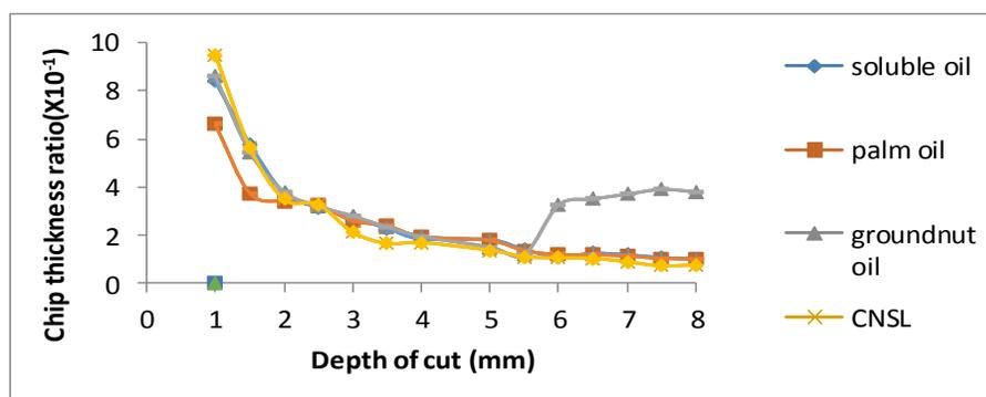
Figure 2: Effect of depth of cut on the chip thickness ratio for mild steel at a constant speed of 150rev/min
