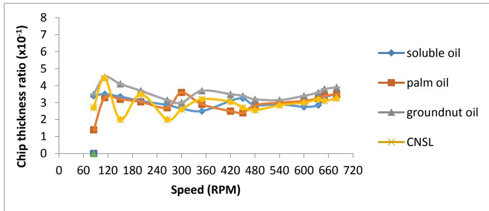
Figure 1: Effect of spindle speed on the chip thickness ratio for mild steel at constant depth of cut of 2mm
