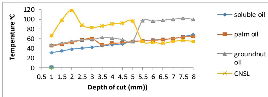
Figure 6: The effect of depth of cut on the temperature for mild steel at a constant speed of 150rev/min
