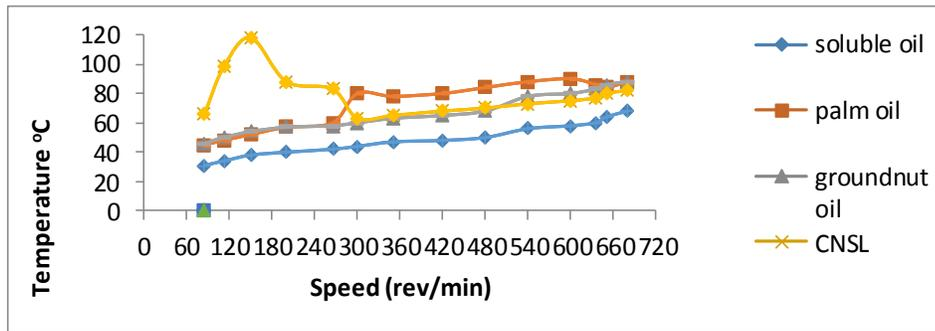
Figure 5: The effect of varying speed on the temperature for mild steel at a constant depth of cut of 2mm
