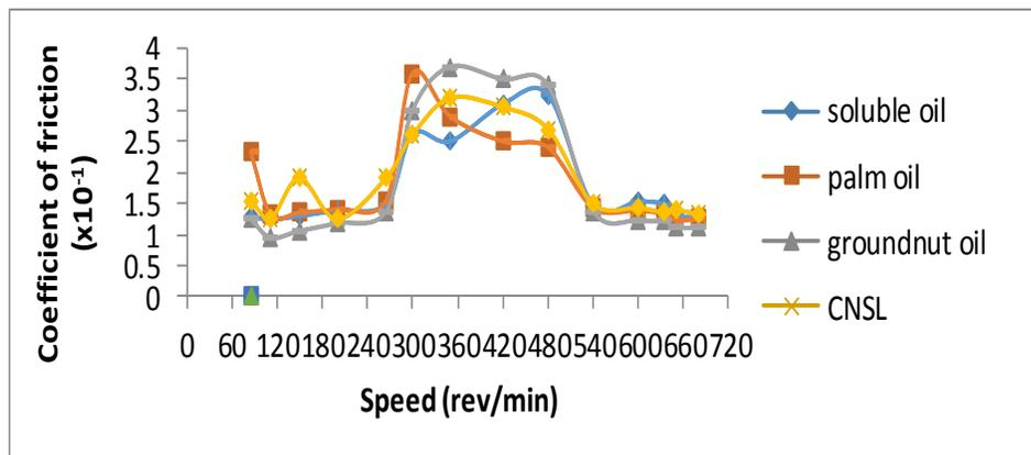
Figure 3: Effect of varying speed on the coefficient of friction for mild steel at a constant depth of cut of 2mm.
