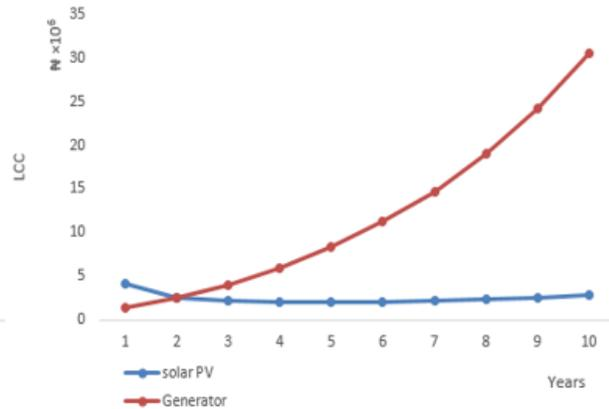
Figure 2: LCC analysis of 5kVA PV and petrol generator.
