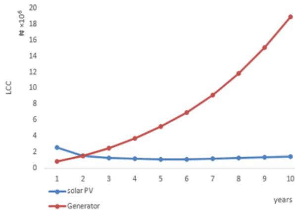
Figure 1: LCC analysis of 3kVA PV and petrol generator.
