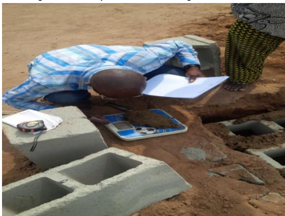
Figure 2: Measurement of Mass of Trowel and Mortar ( M_{Trowel + Mortar} )
