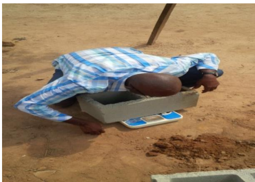
Figure 3: Measurement of Mass of block ( M_{block} )
