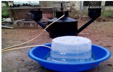
Figure 3. Rear view of the setup for the anaerobic digestion
