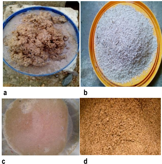
Figure 1. Biomass (raw waste) before and after digestion. Mixed spent grain, rice husk with algae water before digestion (a); Raw rice Husk (b); Digested Slurry (c); Raw brewer spent grain
