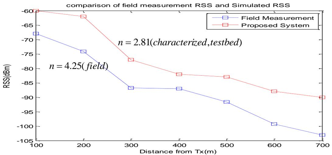
Figure 4. Field path loss exponent (without antenna diversity) compared with pathloss exponent with antenna diversity.
