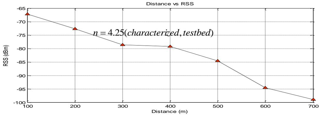
Figure 3. Field data measurement of received signal strength over 100 metres interval distances
