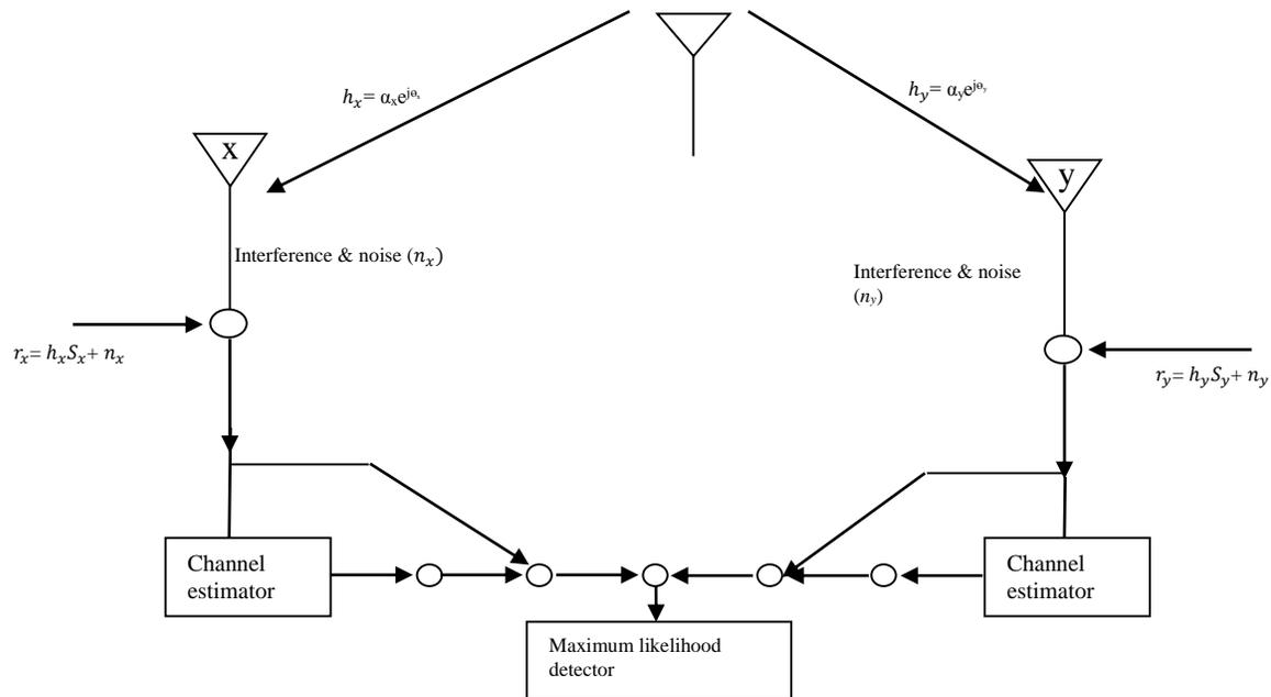
Figure 1. Baseband representation of the classical two-branch MRC
