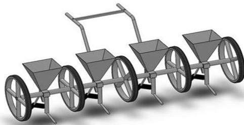
Figure 2. Isometric view of the planter
