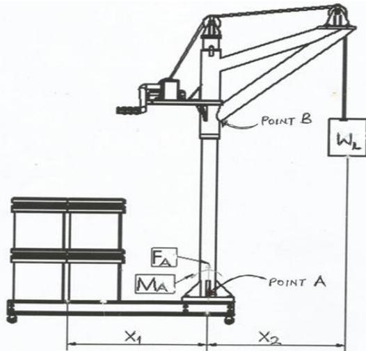
Figure 3: Free Body Diagram of the Crane
