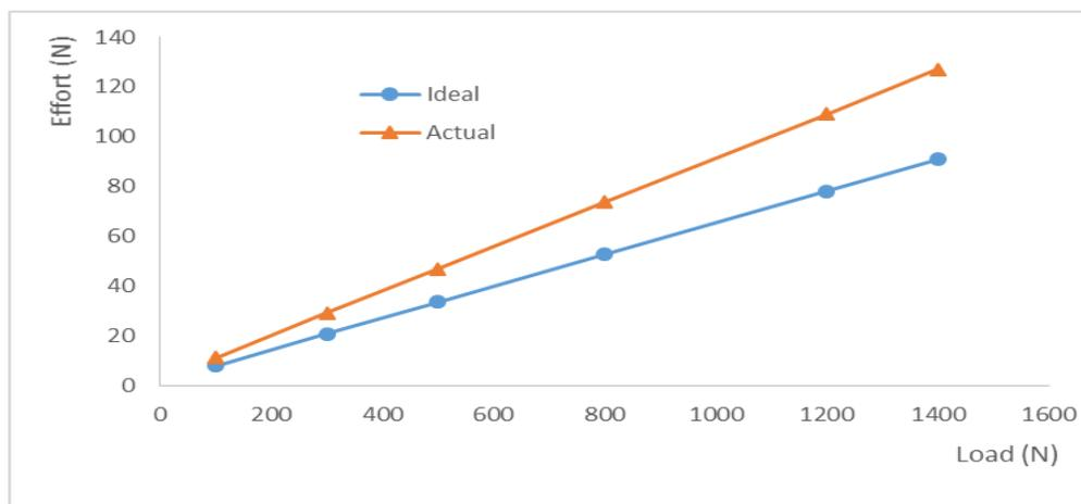
**Figure 11: Mechanical Advantage of the Crane**
