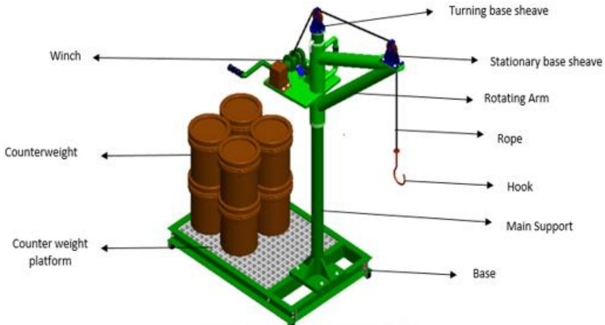
Figure 2: Portable Rotating Arm Balcony Crane
