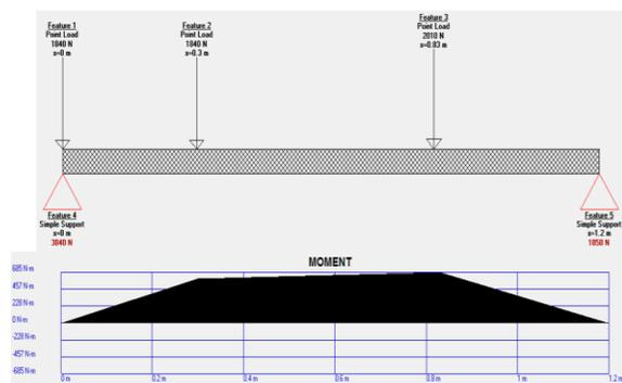
Figure 8: Force Analysis and Bending Moment on the side frame
