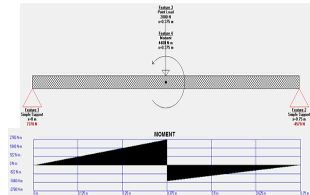
Figure 6: Force Analysis and Bending Moment of the cross piece
