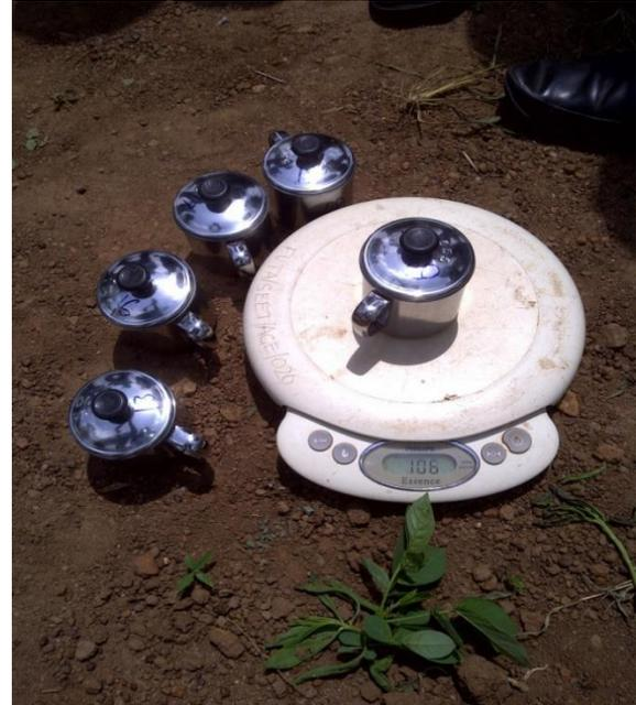
Fig. 1: Plate 1 stainless steel sample containers and weighing Balance
