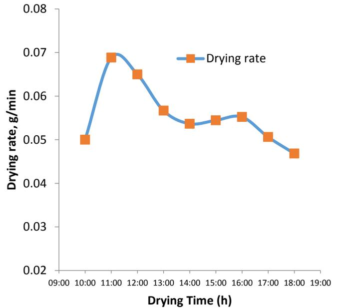
Fig 3b. Drying curve of plantain slices in solar drying
