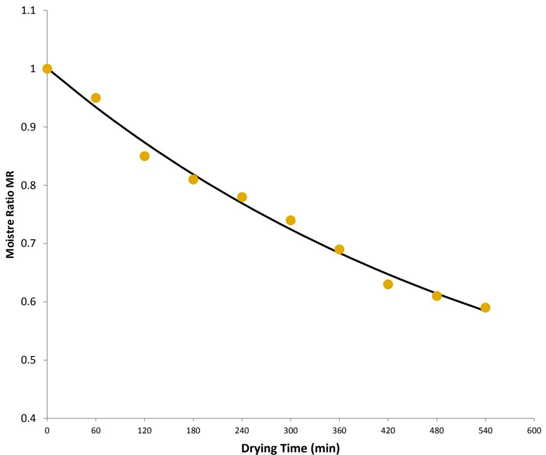
Fig 4. Plot of observed and predicted Moisture Ratio(MR) against drying time of platain slices using Midilli model .
