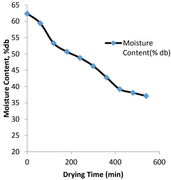
Fig 3a. Drying curve of plantain slices in solar drying
