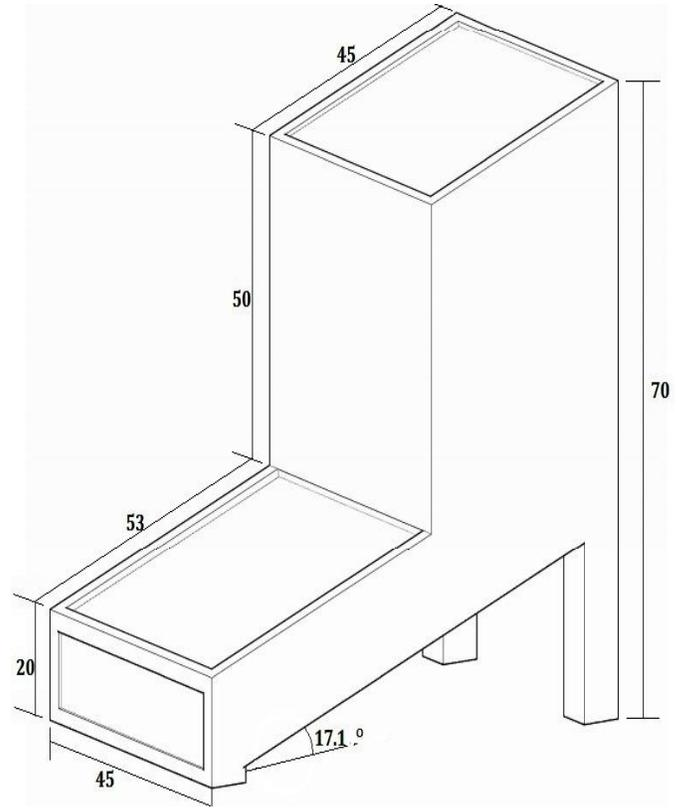
Fig 1. Isometric drawing of the solar dryer
