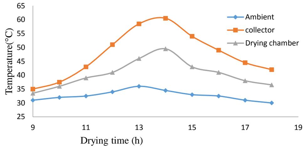
Fig 2 . Hourly temperature variation in the ambient air, solar collector and drying chamber on a typical day during the drying experiment
