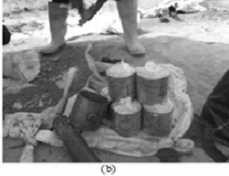
Plate 1: - (a): Complete soaking of compacted samples in CBR moulds with the mounted swell gauges; (b): Split mould, 2.5 kg rammer, and wrapped compacted samples
