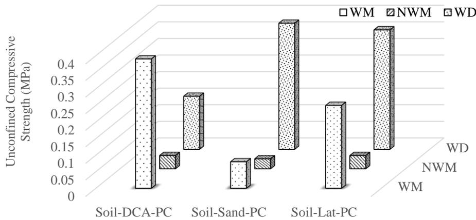
Figure 1: Effect of curing methods on the UCS of samples; WD = Wrapped-dry cured samples; NWM = Not wrapped-moist cured samples; WM = Wrapped-moist cured samples
