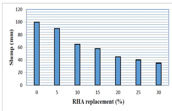
Fig. 2: Variation of slump of the concrete at different replacement levels of RHA.
