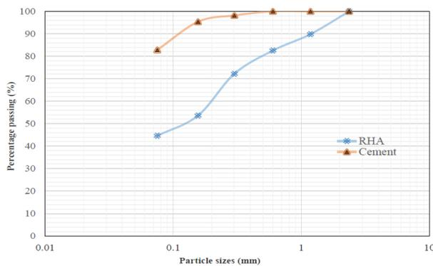
Fig 1c: Sieve Analysis Result of Cement and RHA
