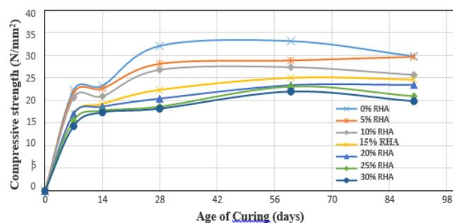
Fig. 5: Variation of compressive strength of Grade 25 concrete with age of curing.
