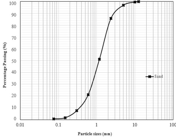
Fig 1a: Sieve Analysis Results of Sand
