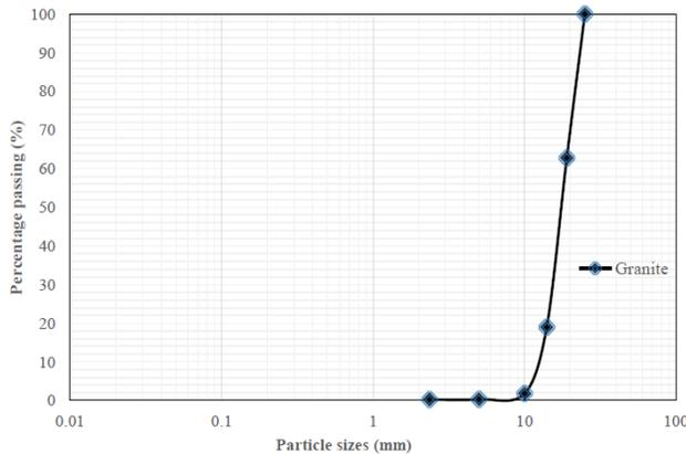
Fig 1b: Sieve Analysis Result of Granite
