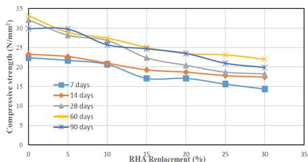
Fig. 4: Variation of compressive strength of Grade 25 concrete with percentage replacement
