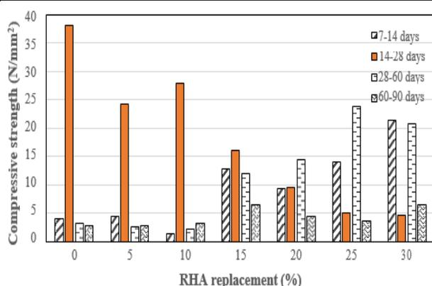
**Fig. 6:** Bar chart showing percentage increase in compressive strength of Grade 25 concrete.
