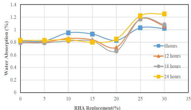
Fig. 3: Variation of water absorption of Grade 25 concrete
