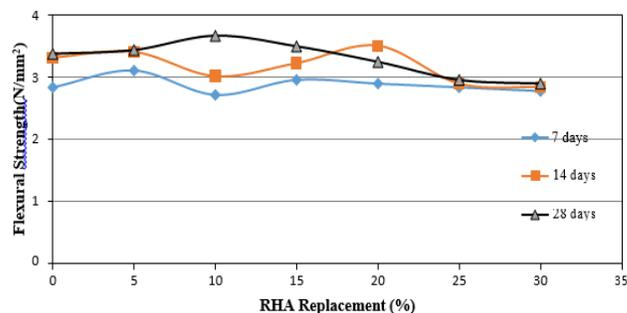
**Fig. 7:** Variation of the flexural strength of Grade 25 concrete beam with age of curing.
