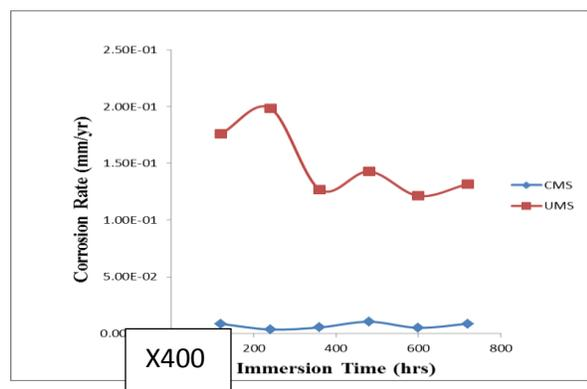
Figure 1: Corrosion rate of CMS and UMS in distilled water against Time
